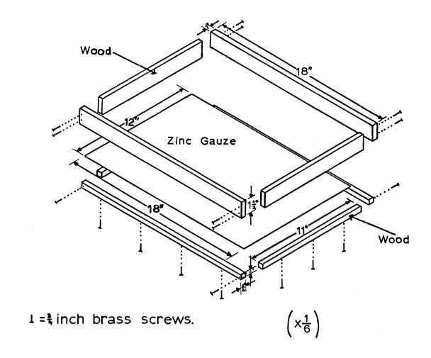
EXPLODED DIAGRAM OF COARSE SIEVE
